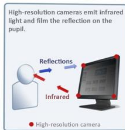
Figure 1: How eye tracking works
